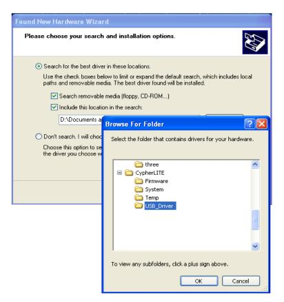
Click "Browse" and select "USB\_Driver" folder in new window, then press"OK" to return last step and by clicking "next" to finish the installation of "USB Drive".
