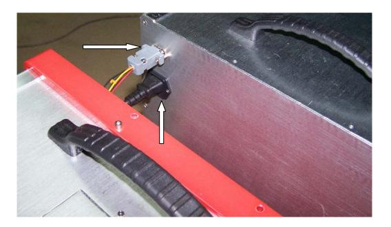
3. Insert laser housing to control housing and then fix joint with screws.
